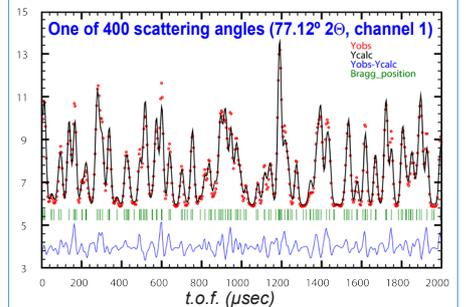
Above: FullProf[3](with POLDI extension) fit of powdered Ge sample, measured with POLDI, including total  $18 \times 8 \times 380 = 54720$  Ge reflections and  $500 \times 400$  data points.
