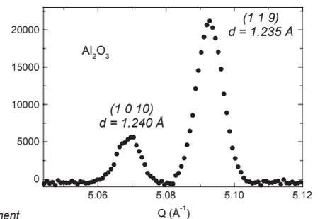
Above: Double peak of  $Al_2O_3$ . The peaks do not even overlap although they are separated by less than 0.5% [2].
