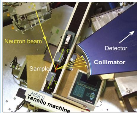
Above: Set-up of an in-situ tensile experiment at POLDI.
