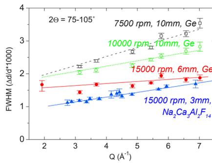
Above: The resolution of POLDI for selected instrument configurations (chopper speed and width of the 2-axis diaphragm). Data points are the result of the correlation method [1].
