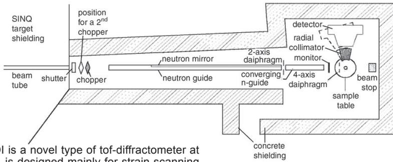
POLDI is a novel type of tof-diffractometer at SINQ, is designed mainly for strain scanning experiments.
