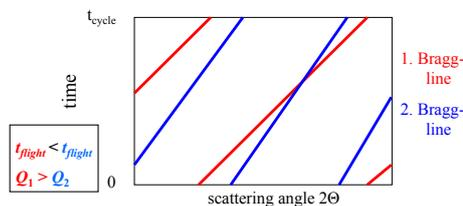
The slopes of the Bragg-lines roughly determine the time-of-flight and therefore also the slit of the chopper the neutrons passed
