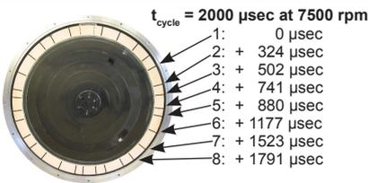
Picture of the chopper disc. The 32 slits are arranged in four identical sequences with pseudo-random distribution.
