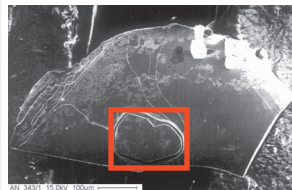
SEM image of a Mg 1-x Fe x B 2 crystal with the inclusion (red area) of the new Mg-Fe-B phase (composition from EDX: \approx Mg 0.75 Fe 0.25 B).
